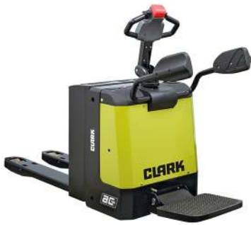
PPX 20 - PALLET TRUCK 2000 Kg
